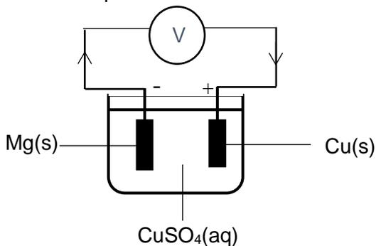
Since **magnesium is more reactive**, the **magnesium metal plate takes the negative electrode where oxidation occurs**:
