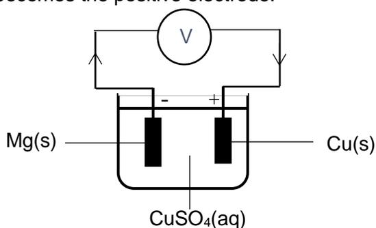
Since **magnesium is more reactive**, the **magnesium metal plate takes the negative electrode where oxidation occurs:**
